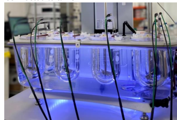
Figure 3: Overall image of 6 arch probes in each vessel with fibre optic cables connected to a PC
